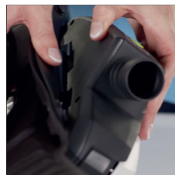
6. Tilt the connecting plate at an angle and slide into place.
