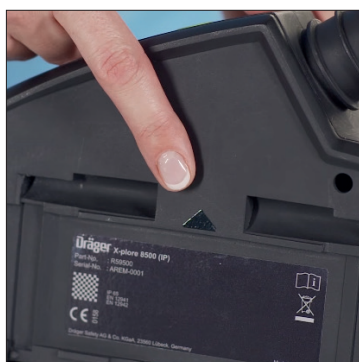
5. Align arrows on the belt and blower unit to match the orientation.
